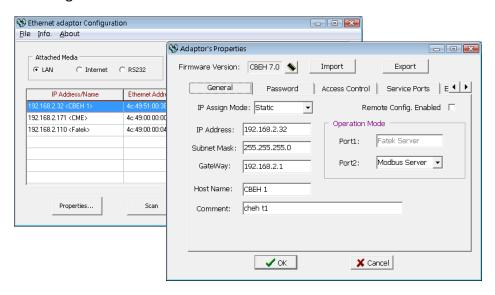
An application that works with the FBs-CBEH series expansion board provides a window-based configuration software, used to set the module's basic settings, password protection and firmware update etc. Please refer to Chapter 3.1 for detailed explanation.
