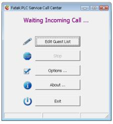
The Service Call Center software is provided to work with remote maintenance operations, used to perform maintenance tasks when the PLC workstation's IP is
