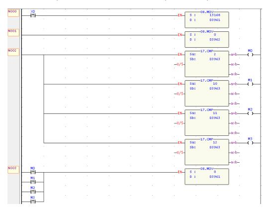
After completing the steps mentioned above, every time X0 changes from 0 to 1, and when D3962 is 0, the mobile phone will receive the SMS sent by the FBs-CBEH series expansion board.
