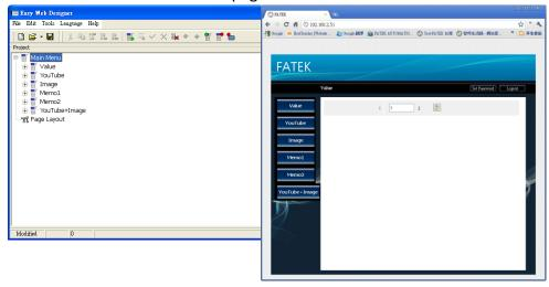
The FBs-CBEH series expansion board provides the function to allow users to easily browse or control the status within the PLC through a customized web page; the customized web page can be created through this software without requiring the user to have the skills to write HTML. Please refer to chapter 4 for detailed explanation.
