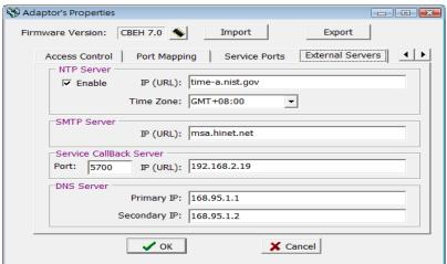
**NTP Server:** The CBEH expansion board provides the internet clock synchronization function, eliminating the trouble of manually correcting the time on a regular basis. To activate this service, just check Enable; when the service is activated, it will periodically request the newest clock data from the NTP server and set the data into Calendar register (D3953~D3960) accordingly (Please refer to Chapter 6 for details).
