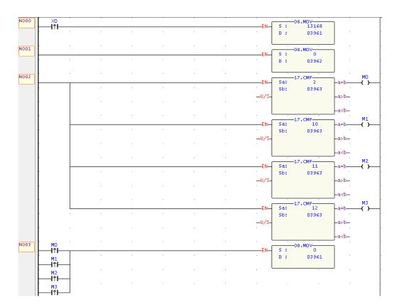
After completing the steps mentioned above, every time X0 changes from 0 to 1, and when D3962 is 0, it will receive the Email sent by the FBs-CBEH series expansion board;
