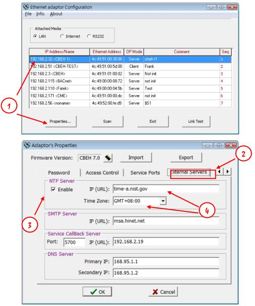
① Move the mouse cursor to the line that includes the CBEH expansion board, double-click it or click the Properties... button to enter configuration setting.
