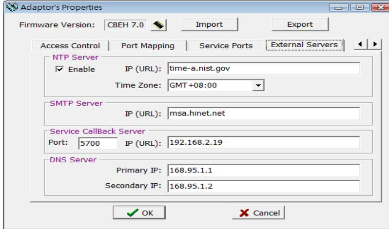
**NTP Server:** The CBEH expansion board provides the internet clock synchronization function, eliminating the trouble of manually correcting the time on a regular basis. To activate this service, just check Enable; when the service is activated, it will periodically request the newest clock data from the NTP server and set the data into Calendar register (D3953~D3960) accordingly (Please refer to Chapter 6 for details).
