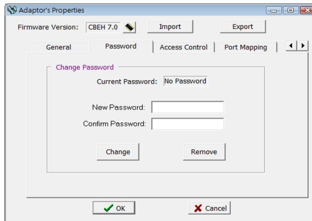
Just enter the password you want to use in the New Password and Confirm Password fields, and then press the Change button to complete the setting. To cancel the password, just press the Remote button.
