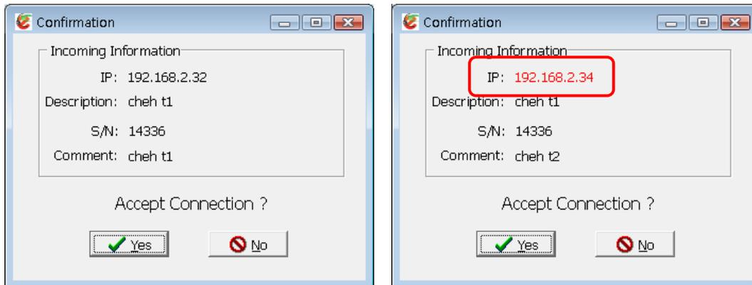
When the connection request window appears, the maintenance personnel can press the **Yes** button to accept this connection or press the **No** button to reject this connection.
