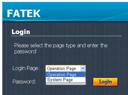
On the login page, users must select the system page from the “login page” combo list and enter the password (**the default factory setting of password is 1234**), then press the **Login** button to log in. If the password is correct, it will enter the system page.
