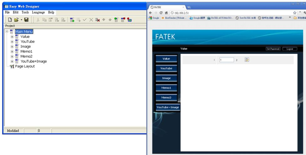
The FBs-CBEH series expansion board provides the function to allow users to easily browse or control the status within the PLC through a customized web page; the customized web page can be created through this software without requiring the user to have the skills to write HTML. Please refer to chapter 4 for detailed explanation.
