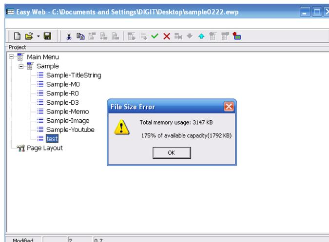
After confirming that the designed webpage content did not exceed the memory capacity provided by the FBs-CBEH series expansion board, click the **OK** button.
