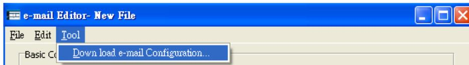
The “Email Configuration transfer” window will appear at this time; in the “Target IP” field, fill in the IP address of the FBs-CBEH series expansion board to download the information, then confirm that the correct password is entered in the “Password” field and press the “Start Download” to perform the downloading.
