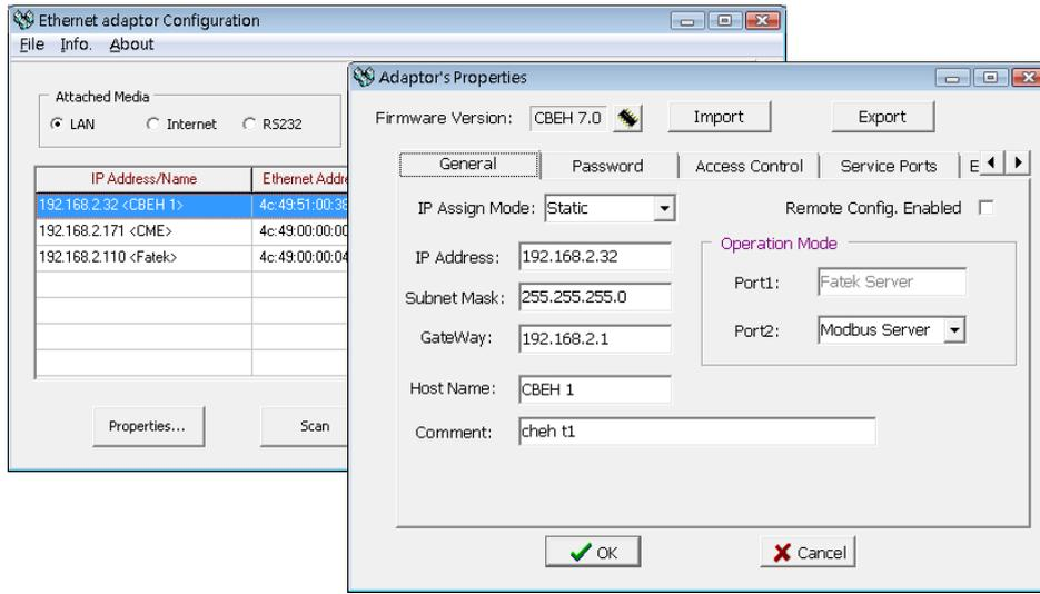
An application that works with the FBs-CBEH series expansion board provides a window-based configuration software, used to set the module's basic settings, password protection and firmware update etc. Please refer to Chapter 3.1 for detailed explanation.
