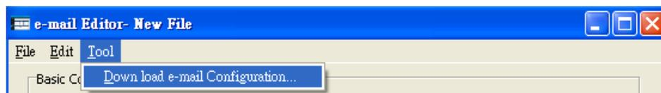
The “Email Configuration transfer” window will appear at this time; in the “Target IP” field, fill in the IP address of the FBs-CBEH series expansion board to download the configuration, then confirm that the correct password is entered in the “Password” field and press the “Start Download” to perform the downloading.
