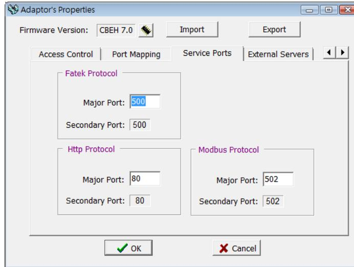
When the CBEH expansion board is working under TCP or UDP server mode, the external service ports must be set so that the external client workstations can send service requests according to the set service port numbers.
