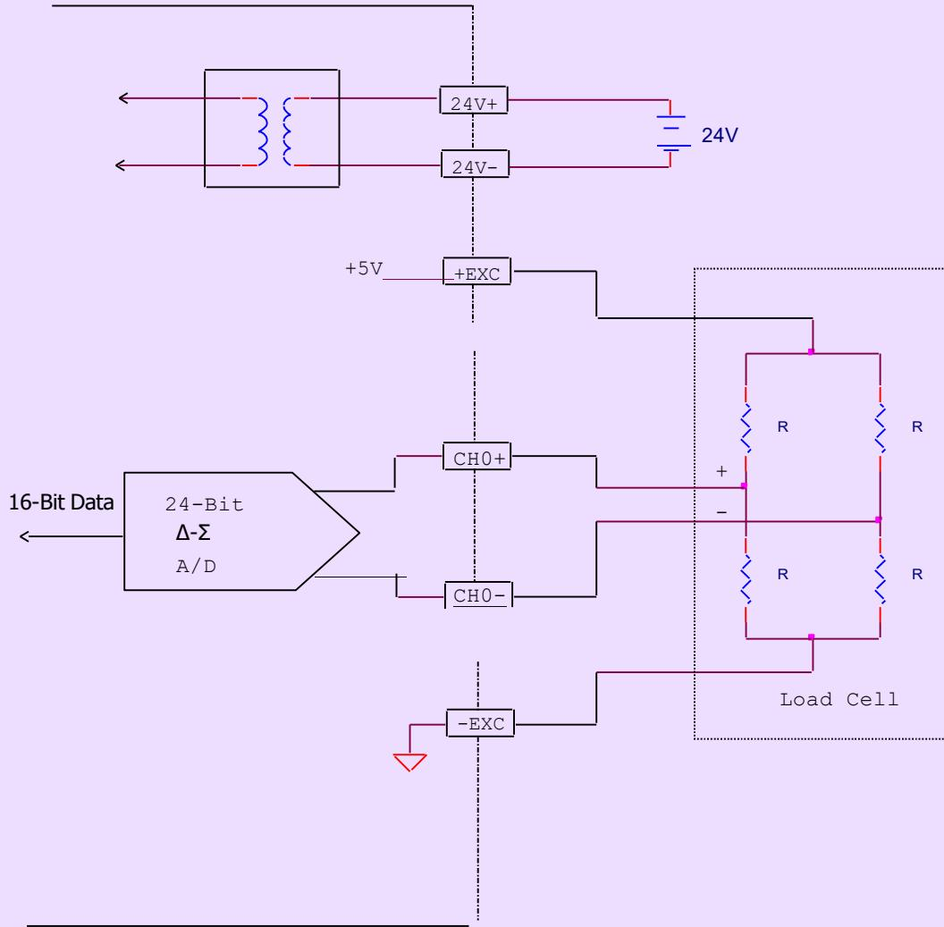
The raw conversion result is represented by a 16-bit signed value. After setting the full range engineering value and perform the zero and full scale calibration procedure, the system will automatically convert the raw conversion reading value into engineering weight value for user application.
