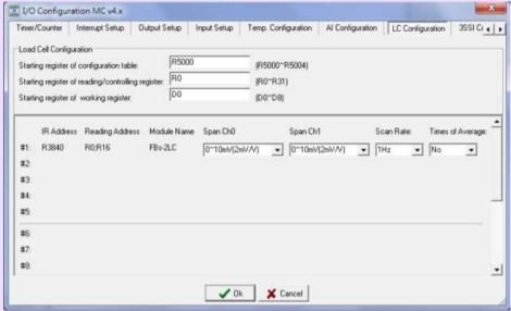
Before FBs-2LC module can be working, the configuration of the module should be set by the Winproladder software tool. The picture shown at above is the I/O configuration page for "LC module" setup.
